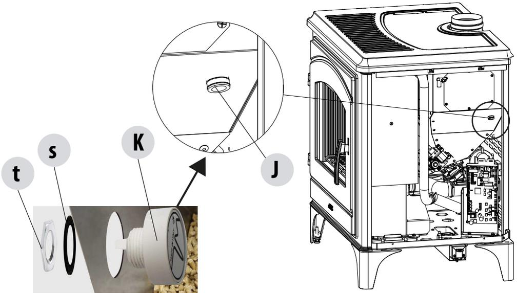
The pellet sensor is a low fuel indicator that warns the user that the pellets are finishing.
